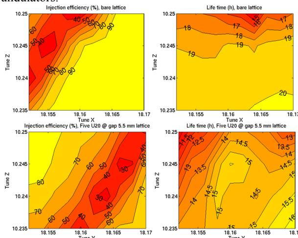
Figure 5: Experimental injection efficiency and beam lifetime scan versus WP with a multibunch 400 mA stored beam.
