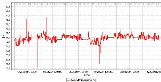
Figure 5: Long-term polarization at the Møller polarimeter (see figure 1) at the final energy.
