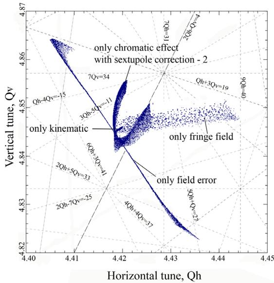
Figure 1: The tune spreads due to each individual effect independently from each other ( $\delta=6\%$ ).
