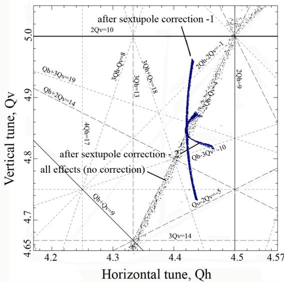
Figure 2: The tune spreads calculated with all sources acting without and with sextupole correction ( $\delta=6\%$ ).
