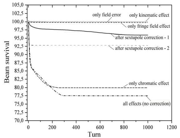
Figure 3: The calculated beam loss in the CR due to different nonlinear sources.
