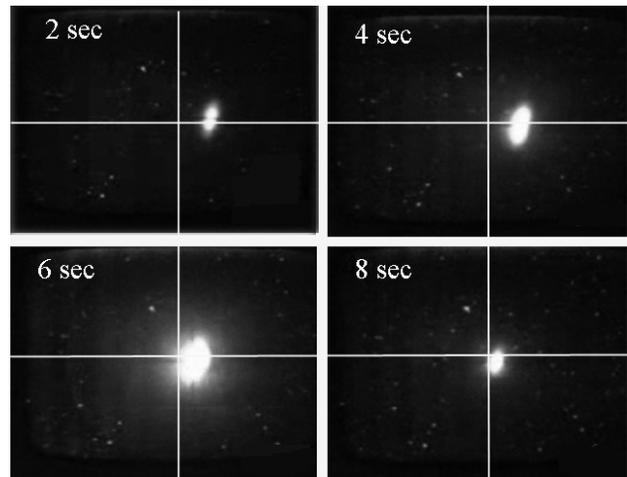
Figure 4: The extracted beam is seen on the illumination screen with a time step of 2 seconds.
