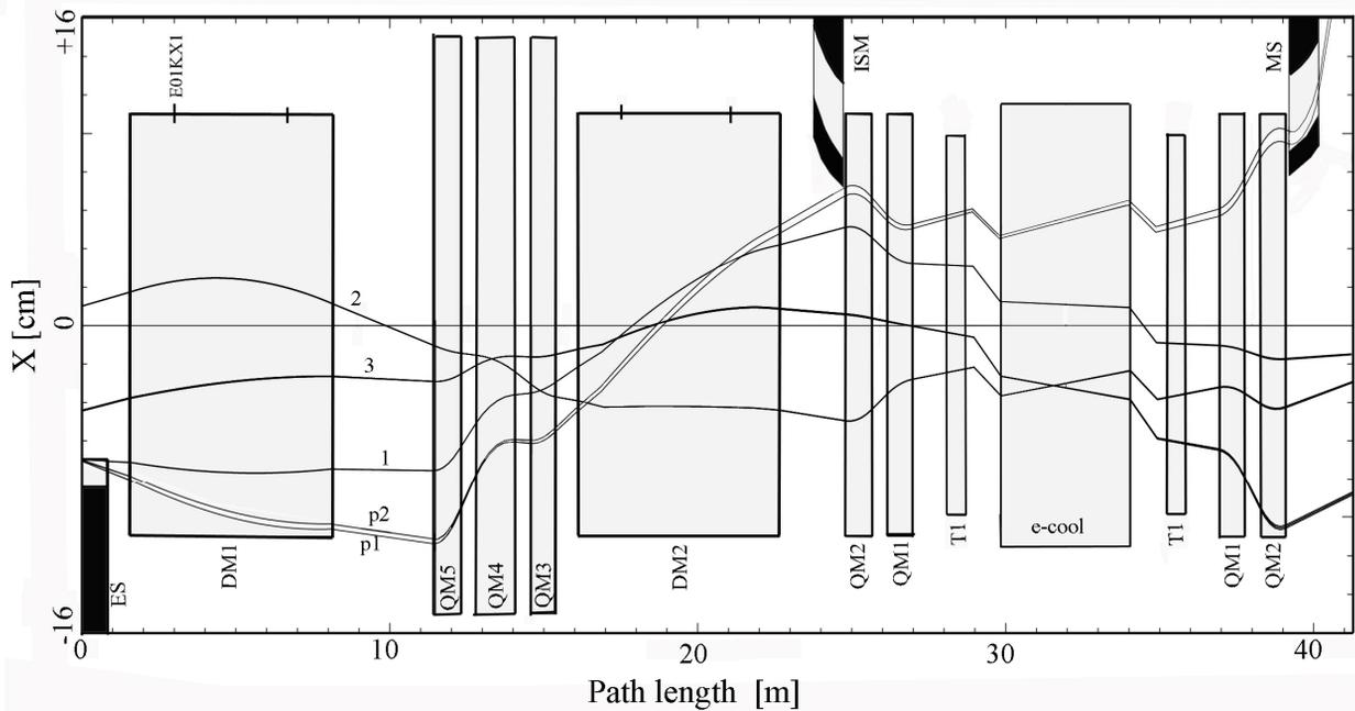
Figure 1: Particle trajectories in the region from the Electrostatic Septum (ES) to the Magnetic Septum (MS). ISM – Injection Septum Magnet, e-cool –electron cooler, DM–Dipole Magnet, QM–Quadrupole Magnet, E01KX1 – corrector magnet. Boxes show the limit of beam survival with real aperture limitations. Numbers 1,2,3 correspond to the last three turns in the ring; p1,p2 – trajectories of the kicked particles by the ES with the initial angle  $\Delta x_1'$  and  $\Delta x_2'$  ( Fig.2).
