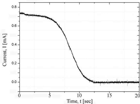
Figure 3: The beam current in the ring during moving of the horizontal tune to the resonance 7/3.
