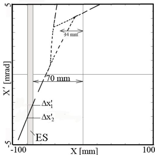
Figure 2: The phase space at the entrance of the ES.  $\Delta x_1'$  and  $\Delta x_2'$  are the initial angles of particles before they are kicked by ES and directed to MS as shown in Fig.1.
