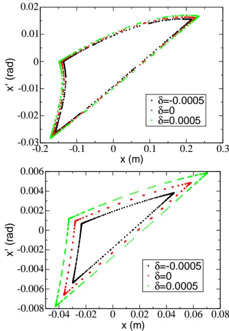
Figure 1: Stable phase areas for  $\delta = -\sigma_p, 0, +\sigma_p$  with  $\sigma_p = 5 \times 10^{-4}$  from Table 1 at  $\nu_x = 4.27$  (graph above) and  $\nu_x = 4.32$  (graph below). Note the different axis scales.
