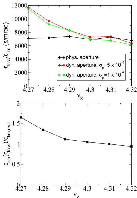
Figure 3: Loss times  $\tau_{loss}$  normalised to the acceptance  $\epsilon_{lim}$  for physical and dynamic aperture (graph above) and dynamic aperture calculated from the loss times according to Eq. (5) (graph below).
