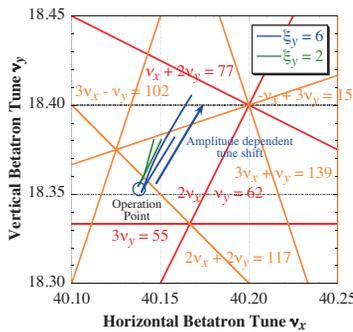
Figure 7: Tune excursion of the betatron tune with the growing amplitude in the tune map.
