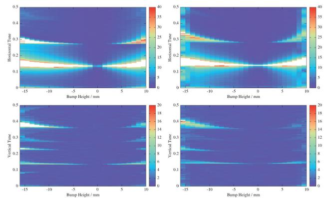
Figure 5: Fourier transform of beam oscillation after kicked by pulse bump magnets.
