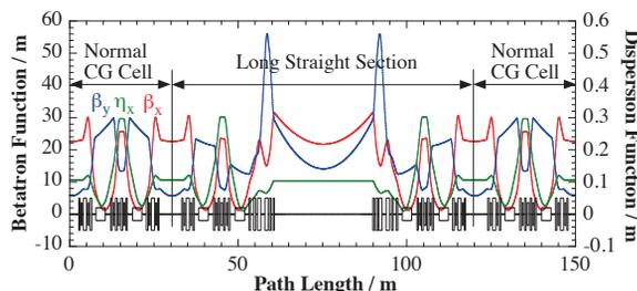
Figure 2: Lattice functions of low emittance optics of the SPring-8 storage ring. The red (blue) line denotes the horizontal (vertical) betatron function and the green one represents the horizontal dispersion function.
