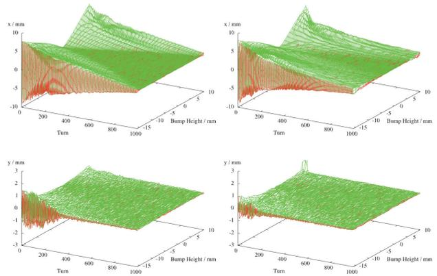
Figure 4: Beam oscillation in time domain after kicked by pulse bump magnets.
