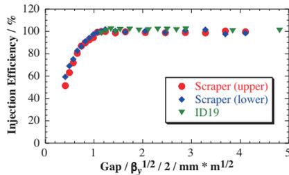
Figure 3: Injection Efficiency vs. scraper gap.
