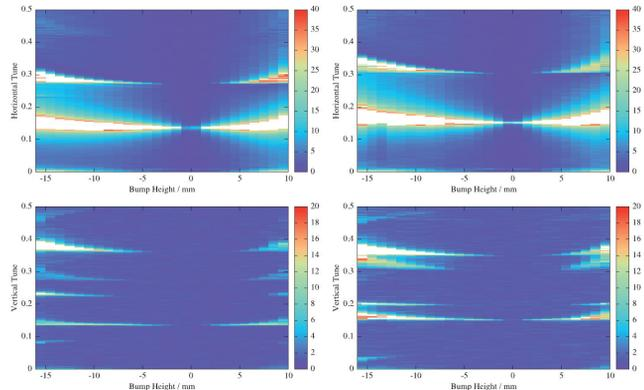
Figure 8: Fourier transforms of beam oscillation of operation point  $(40.14, 18.35)$  (left) and  $(40.15, 18.35)$  (right). Figures at upper (lower) line represent the horizontal (vertical) oscillation.
