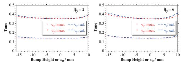
Figure 6: Comparison of the measured amplitude dependent tune shift with the simulation.
