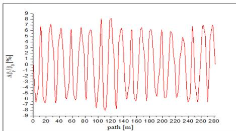
Figure 3: Change in the vertical betatron function caused by Ids without corrections.
