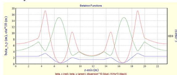
Figure 2: Betatron functions in horizontal (red solid line), vertical (green solid line) planes and dispersion function (blue solid line).
