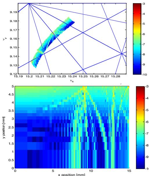
Figure 9: Frequency map in frequency (upper) and coordinate (bottom) spaces for  $Q_x = 15.243$  and  $Q_y = 9.181$  with non-linear intrinsic and horizontal field roll-off after the iterative Twiss and tunes matching.
