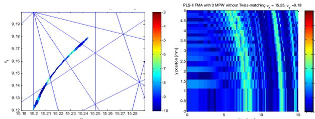
Figure 1: Diffusion map for the PLSII lattice with horizontal and vertical tunes of 15.245 and 9.18, respectively.
