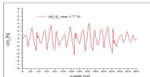
Figure 7: Variation of betatron function for  $Q_x = 15.243$  and  $Q_y = 9.181$  with three wigglers and eight in-vacuum undulators after Twiss matching and storing tunes.
