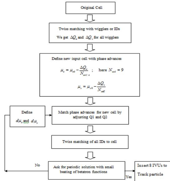
Figure 6: Flow diagram for iterative Twiss while keeping the tunes close to design values.
