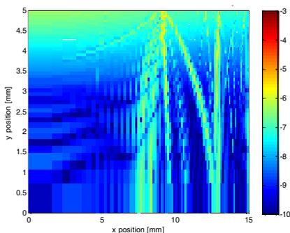
Figure 8: Diffusion map in coordinate space for the PLSII lattice ( $Q_x = 15.243$  and  $Q_y = 9.181$ ) with intrinsic nonlinear fields of three wigglers and eight IVU20.
