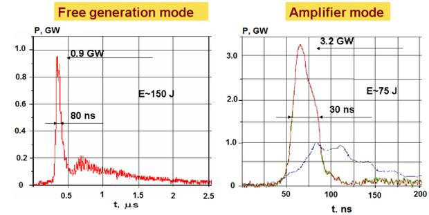
Figure 3: Pulses of L100 laser radiation for auto-generator and amplifier modes of operation.
