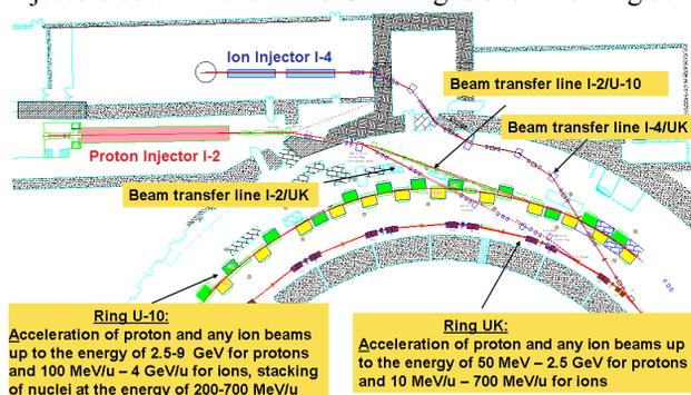
Figure 5: Project of ITEP-TWAC Injection Complex.
