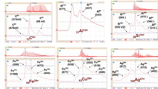
Figure 4: Ions generation in LIS with laser L100.
