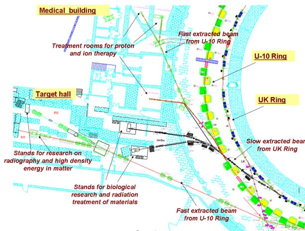
Figure 6: Layout of experimental area for applications.
