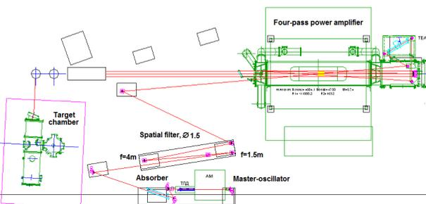
Figure 2: Optical scheme of LIS in amplifier mode.
