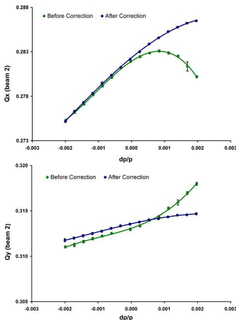
Figure 1: Nonlinear chromaticity of Beam 2 before and after the  $Q''$  and  $Q'''$  corrections were applied to the MCO and MCD spool pieces.
