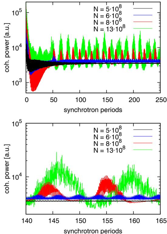
Figure 1: Time dependent emission of coherent radiation for different numbers of electrons per bunch. The bottom graph shows a close-up example of the longtime dynamics.
