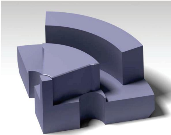
Figure 2: 1/8 model of designed magnet.
