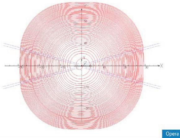
Figure 6: The single particle track of compact cyclotron.
