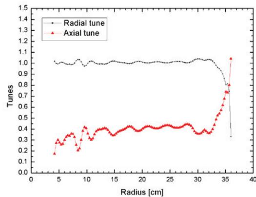
Figure 4: Radial and axial beam tunes.
