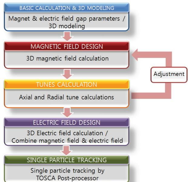
Figure 1: Steps of simulation process.
