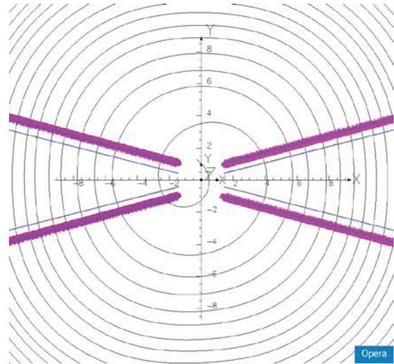
Figure 7: Radial trajectories of single particle for the first 8 turns with electric field vectors.
