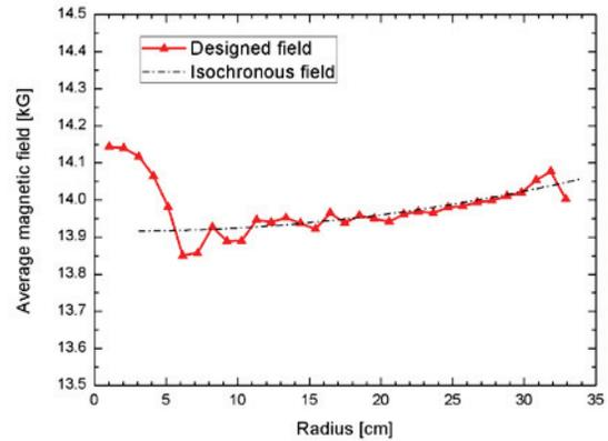
Figure 3: Average magnetic field along the average radius.
