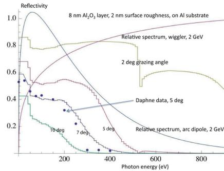
Figure 1: An example of the reflectivity of photons on a specified surface. Data was taken from the Berkeley Center for X-Ray Optics [4] and Daphne [7]. Plot courtesy of G. Dugan.
