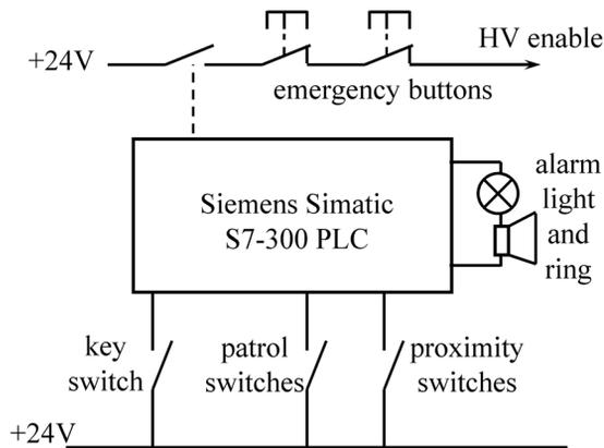
Figure 4: Schematic of interlock system.
