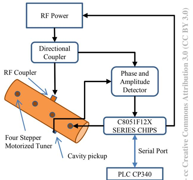
Figure 1: Layout of the AFC and AGC system.
