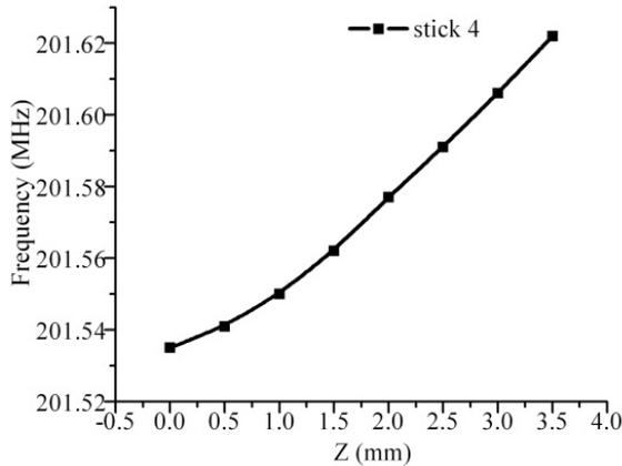
Figure 2: Frequency shift caused by the fourth stick tuner
