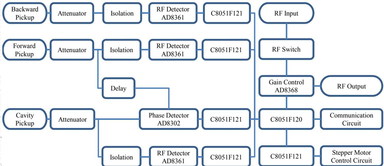
Figure 1: Schematic of AFC/AGC circuit board.
