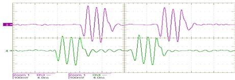
Figure 2: Horizontal and vertical Front-End output doublets.
