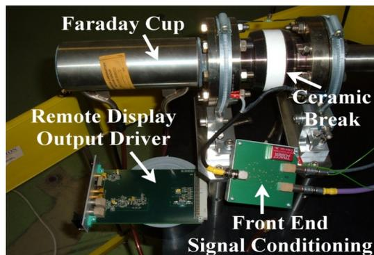
Figure 5: Faraday Cup and its Front-End together with an Output Driver.
