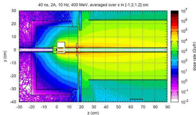
Figure 2: simulation of radiation field near teststand at DESY LINAC II converter (FLUKA 2011[9][10]).
