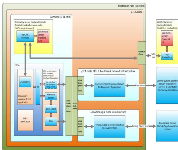
Figure 1: XFEL machine dosimetry system integration into MPS- and Control System environment.
