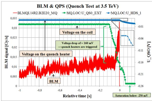
Figure 3: Comparison of signals during the quench. Red line – BLM, green line – voltage difference between apertures, blue line – voltage on quench heaters.
