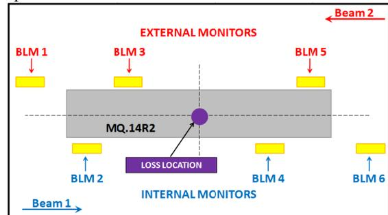
Figure 5: Each MQ is equipped with six monitors, - the three external BLMs (with respect to the LHC ring centre) survey beam 2 while the three internal detectors observe beam 1.
