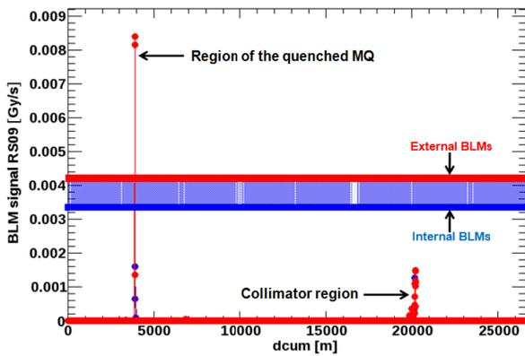
Figure 4: Beam losses along the LHC ring.
