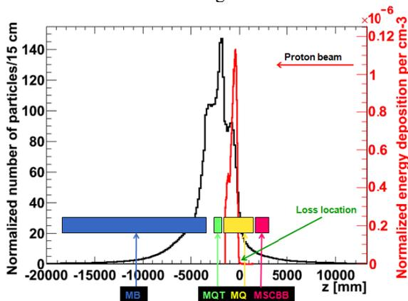
Figure 6: Energy deposition along a coil cable (for a region where  $E_{dep}$  reaches a maximum) and the number of particles registered outside the cryostat. Main magnets have been marked.
