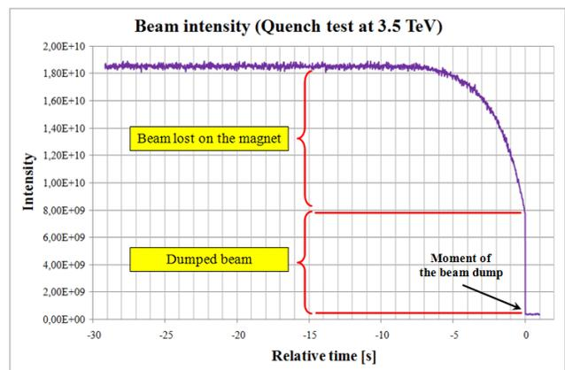
Figure 2: Beam intensity of the 3.5 TeV proton beam during the quench test as provided by the Beam Current Transformer (BCT).
