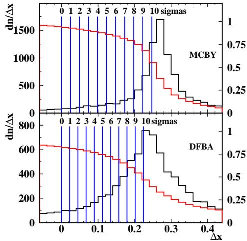
Figure 3: Projection along the  $x$  axis of the distribution of protons that are going to interact with some element along the line within cell C13.R6, at the exit of the MCBY.5R6 (top) and of the DFBAL.5R6 (bottom). The normalized cumulative, from outside to inside, is shown in red. The corresponding number of sigmas from the ideal trajectory is shown by means of blue lines.
