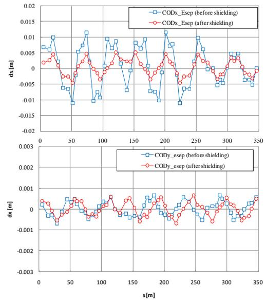
Figure 6: Horizontal and vertical COD measurements at 181MeV storage mode where the ESEPs excited at 3GeV.
