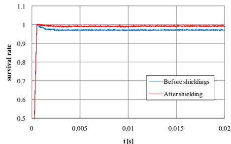
Figure 8: The beam survival rate at 3GeV acceleration mode was measured before and after additional shielding.
