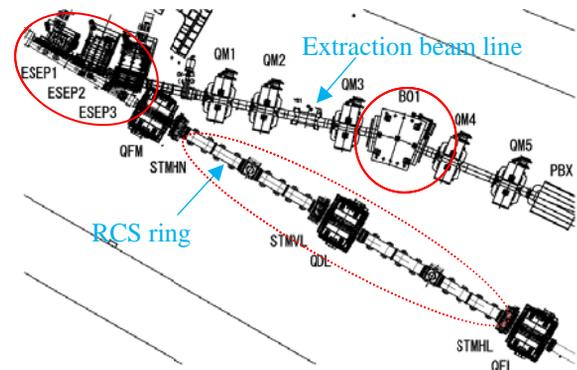
Figure 1: The schematic diagram of the RCS extraction area.
