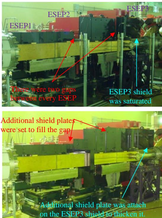
Figure 4: Photo of the ESEPs assembled with the additional shield plates. Upper and lower shows the comparison between before and after shielding.
