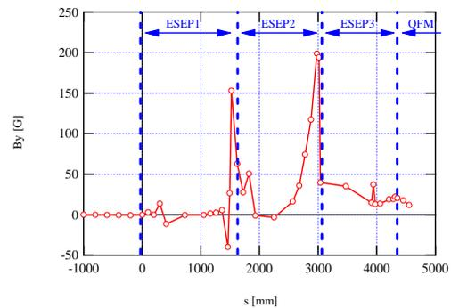
Figure 2: Measured leakage field distribution from the ESEPs along the s-axis on the top of the vacuum chamber, in which the origin of s-axis indicates the upper-stream flange of the ESEP1.
