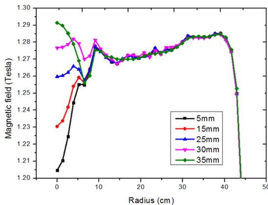
Figure 6: Magnetic fields change the height of variable part in centre pole.
