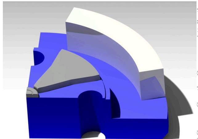
Figure 1: 1/8 Model of 13MeV Magnet.
