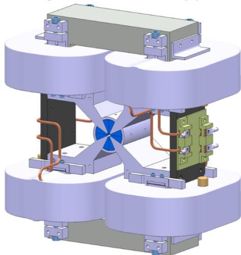
Figure 4: View of the Short QD0 Prototype.
