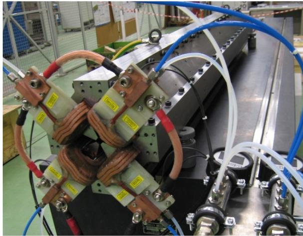
Figure 2: The assembled type4 MBQ magnet.
