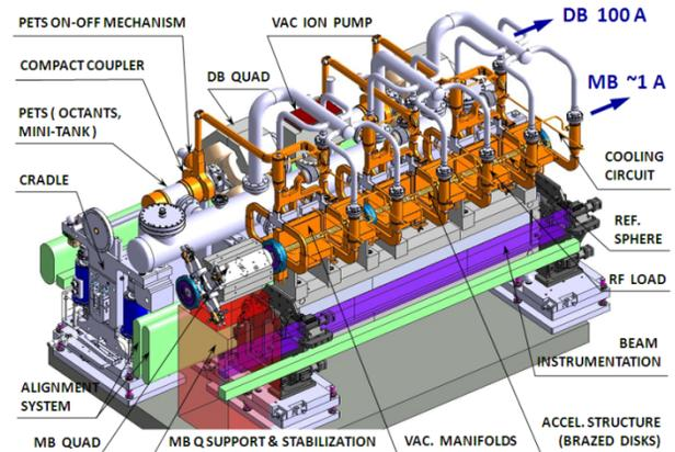
Figure 1: View of a typical CLIC Module.
