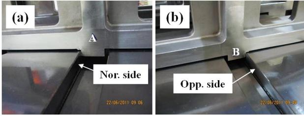
Figure 2: The feet installation of magnet in the two-side measurement. The marker A and B are the different side of magnet.
