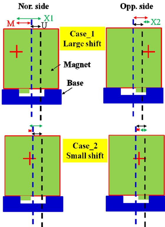
Figure 3: An exaggerated sketch of the two-side measurement of the large and small offsets.
