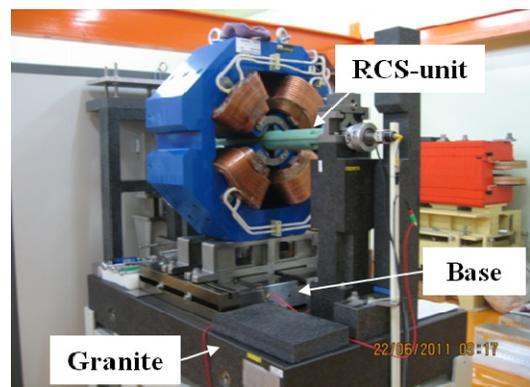
Figure 1: The photograph of RCS. The RCS-unit support and magnet base are mounted on a granite bench.
