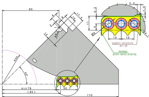
Figure 4: Lamination of the 3 Turn quadrupole
