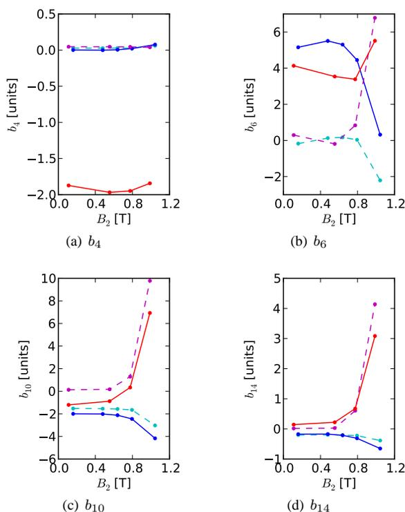
Figure 5: Comparison of the central and the total field quality of the 3 turn (central — dashed cyan line, total solid blue line) to the 6 turn (central — dashed magenta line, total solid red line)
