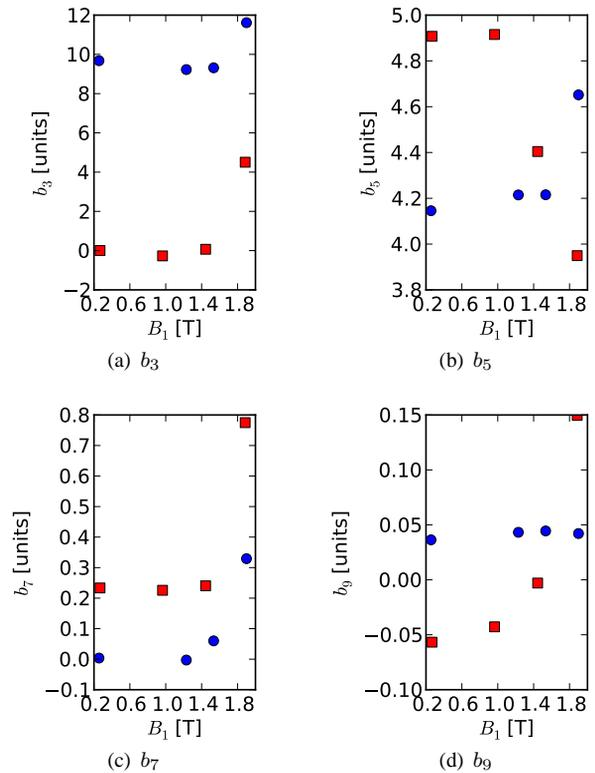
Figure 3: Influence of the insert on the field quality. Blue... original design, red... optimised shape.
