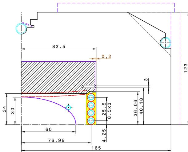
Figure 1: The sextupole superimposed on the pole surface of the SIS100 dipole lamination. The hatching indicates the insert. The red dashed line indicates the superimposed sextupole shape.
