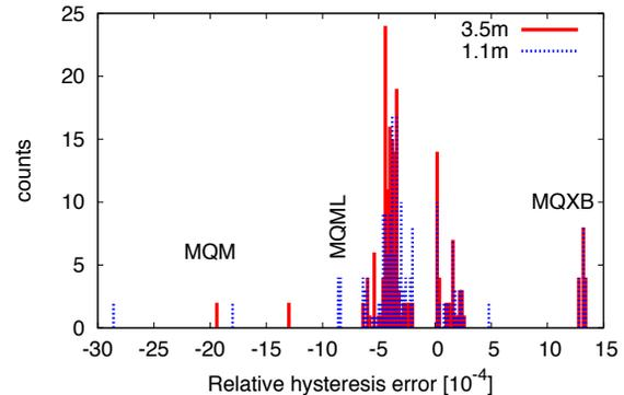
Figure 5: Hysteresis errors seen from quadrupoles used during optics squeeze at  $\beta^* = 3.5$  m and 1.1 m.
