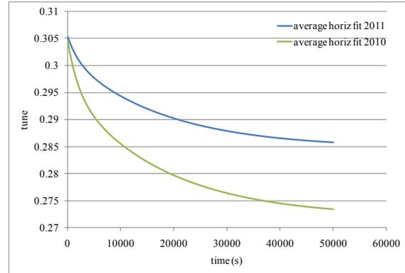
Figure 3: Difference between 2010 and 2011 of the average horizontal tune decay during injection.
