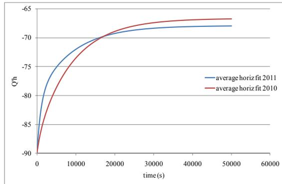
Figure 4: Difference between 2010 and 2011 of the average horizontal chromaticity decay during injection.
