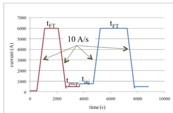
Figure 1: Current pre-cycle and cycle used for the LHC main dipoles and quadrupoles since September 2010.
