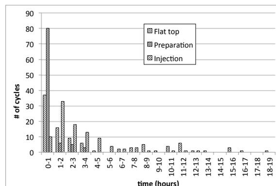
Figure 2: Histogram of time spent during the flattop, preparation and injection over 96 cycles in 2011.
