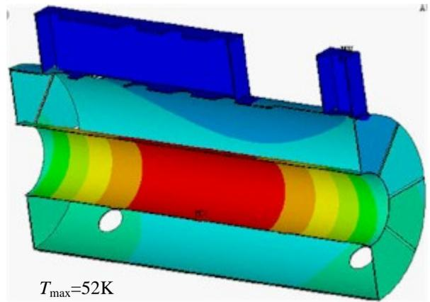
Figure 8: Radiation shield temperature distribution.
