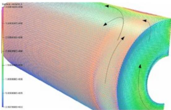
Figure 6: Radiation shield eddy current analysis.
