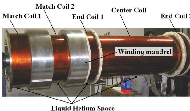
Figure 3: Spectrometer solenoid cold mass assembly.
