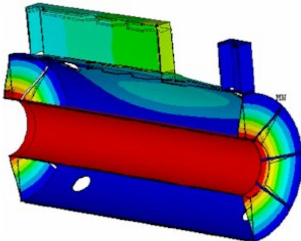
Figure 7: Radiation shield displacements during shipping.
