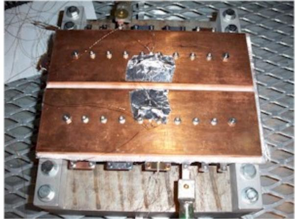
Figure 4: Test of the resistor conductive cooling scheme.
