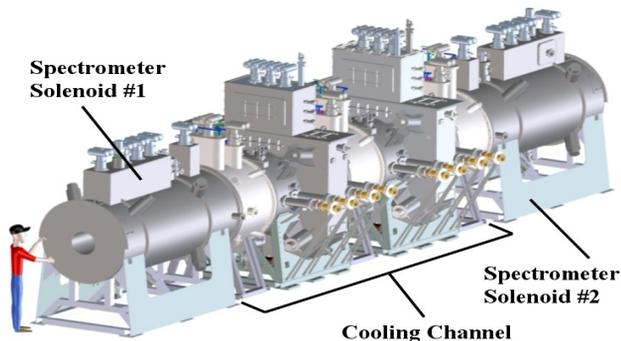
Figure 1: MICE cooling channel 3D CAD image.
