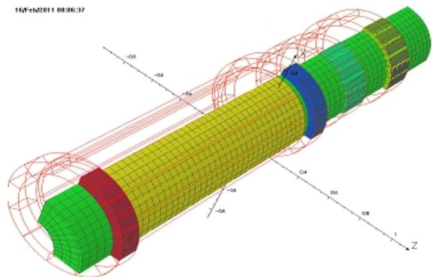
Figure 5: 3D quench analysis model.
