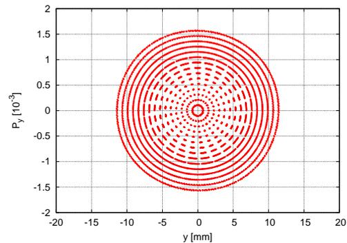
Figure 6: Tracking of a particle with the initial vertical position  $n\sigma_y$  at the injection point, the other positions are set to zero and  $n$  varies from 1 to 15 with an increment of 1.
