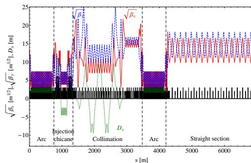
Figure 2: Horizontal betatron function (red full line), vertical betatron function (blue dashed line) and horizontal dispersion (green dotted line) in the whole DR.
