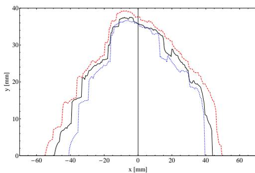
Figure 4: Dynamic aperture at the center of the injection insertion for 10,000 turns at  $\delta = 0, 0.25, -0.25\%$  (black full line, red dashed line and blue dotted line).
