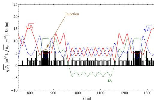
Figure 3: Horizontal betatron function (red full line), vertical betatron function (blue dashed line) and horizontal dispersion (green dotted line) in the injection chicane.
