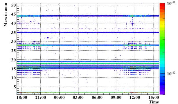
Figure 1: The residual gas spectrum in a synchrotron is changed by the desorbed gases. During high current operation (left and right), additional components appear with a density comparable with the static background spectrum. The gap in between indicates the time of low intensity operation.
