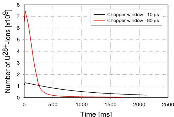
Figure 3: First experiments with  $U^{28+}$  in SIS18 in the year 2001. Ionization processes in sections where the pressure was enhanced by ion induced desorption, caused an almost complete loss of the beam.
