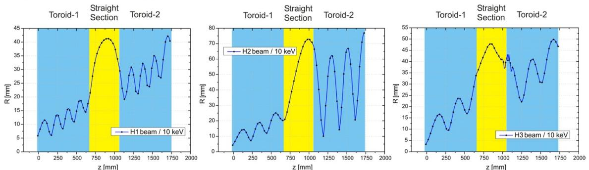
Figure 6: Center of beam motion as a result from PIC-simulation for  $H^+$ ,  $H_2^+$  and  $H_3^+$  species (from left to right) along the toroidal transport section.
