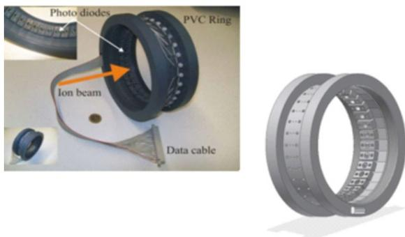
Figure 8: Optical diagnostic probe. Photodiodes are arranged on a cylindrical ring.
