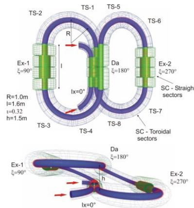
Figure 2: The Figure-8 low energy storage ring with guiding magnetic field.
