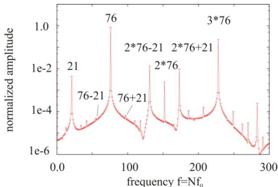
Figure 3: Basic frequencies and their harmonics for magnetic flux structure.
