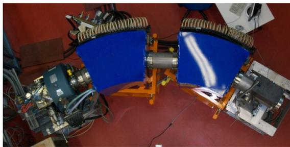
Figure 4: View on the setup of the toroidal beam transport experiment.
