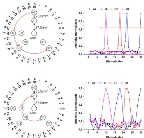
Figure 9: Position of test probe in a cylindrical geometry and corresponding photodiode signals.
