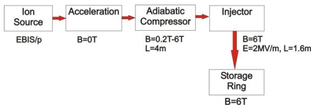
Figure 1: General view of an injection scheme.
