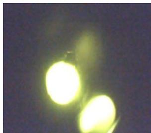
Figure 7: Separation of  $H^+$  and  $H_2^+$  parts of the composite beam at the end of the toroidal transport section.
