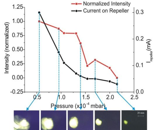
Figure 5: Dependence of measured beam profile on buffer gas pressure.
