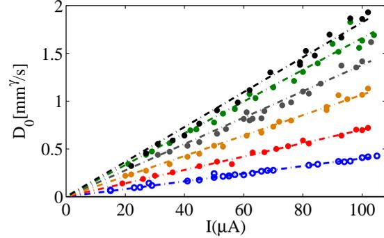
Figure 3: Measured heating terms  $D_i$  of coasting (blue) and bunched  $^{12}\text{C}^{6+}$  ion beams as a function of intensity. At resonator voltages of  $46.5 \text{ V}$  (red),  $93.0 \text{ V}$  (yellow),  $139.5 \text{ V}$  (grey),  $186.5 \text{ V}$  (green) and  $232.5 \text{ V}$  (black) the heating term of bunched ion beams were measured.
