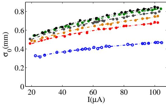
Figure 4: Measured horizontal equilibrium beam width as a function of intensity for  $^{12}\text{C}^{6+}$  coasting (blue) and bunched ion beams. At resonator voltages of 46.5 V (red), 93.0 V (yellow), 139.5 V (grey), 186.5 V (green) and 232.5 V (black) the equilibrium beam widths of the bunched ion beams were measured.
