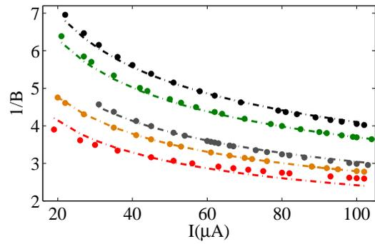
Figure 5: Inverse bunching factor for different resonator voltages as a function of the beam intensity. At resonator voltages of 46.5 V (red), 93.0 V (yellow), 139.5 V (grey), 186.5 V (green) and 232.5 V (black) the inverse bunching factor of bunched ion beams were measured.
