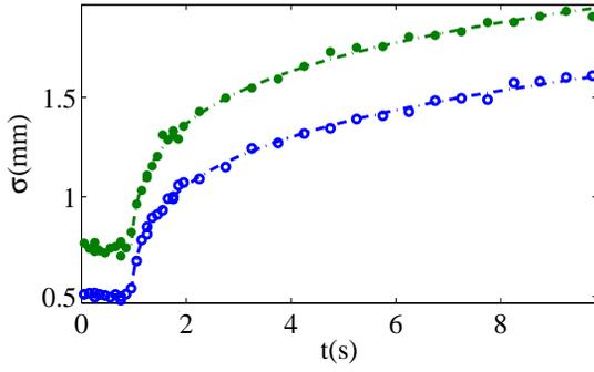
Figure 1: Measured horizontal beam width as a function of time for  $^{12}\text{C}^{6+}$  coasting (blue) and bunched (green) ion beams.
