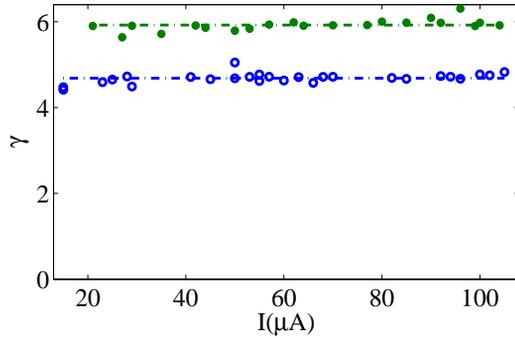
Figure 2: Measured  $\gamma$  parameter for  $^{12}\text{C}^{6+}$  coasting (blue) and bunched (green) ion beams as a function of the beam intensity.
