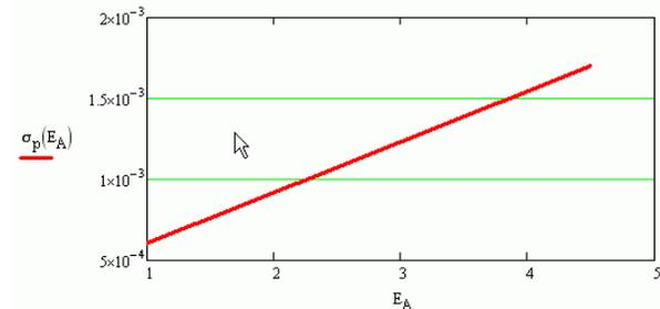
Figure 3: Momentum spread vs. ion energy in collision mode.
