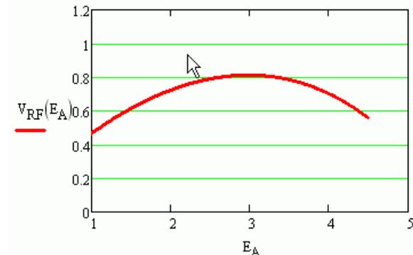
Figure 4: RF3 amplitude (MV) vs. ion energy (GeV).
