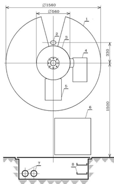
Figure 5: Preliminary design of RF station for 2<sup>nd</sup> and 3<sup>rd</sup> RF systems.
