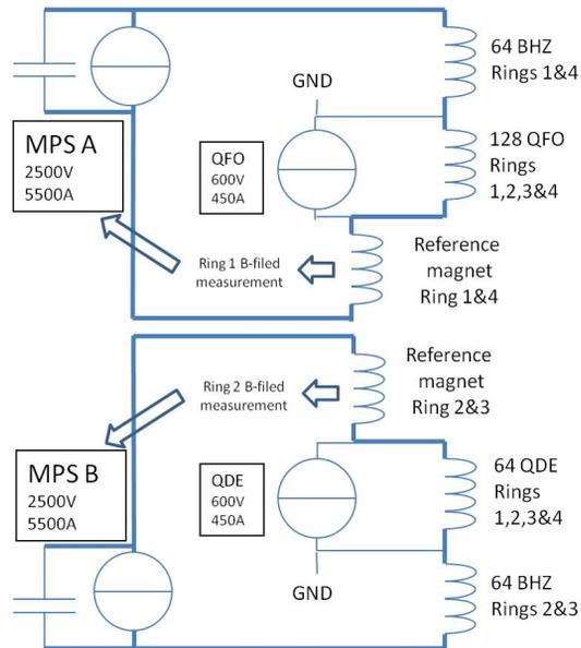
Figure 2: Lay-out of new POPS-type main power supply.
