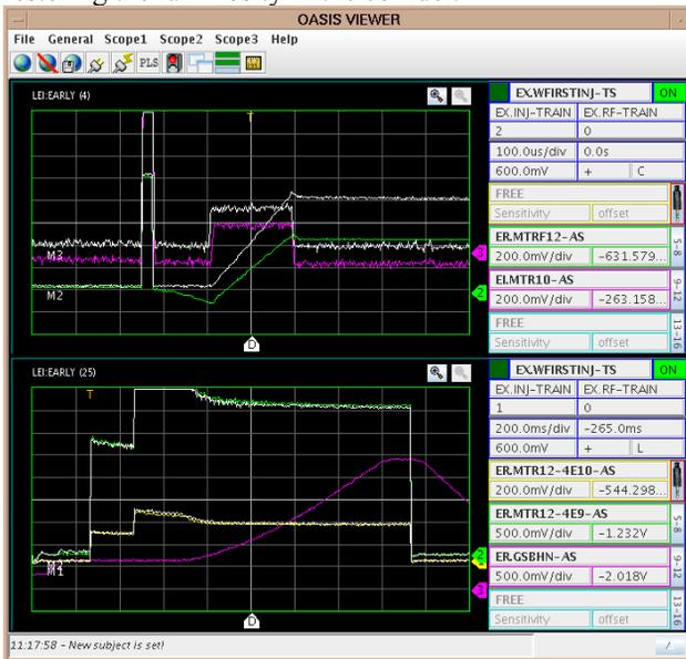
Figure 1: Double injection into LEIR. The top screen shows the first (white) and second (colour) Linac pulses in the transfer line and accumulated in the ring. The lower screen shows the particle current (yellow/green) and the magnetic cycle (magenta); the flat bottom was lengthened to allow enough time for electron cooling of the particles after the second injection.
