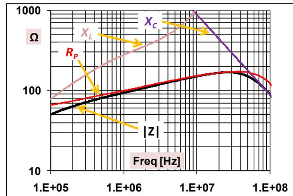
Figure 2: Response of a Finemet<sup>®</sup> loaded resonator.
