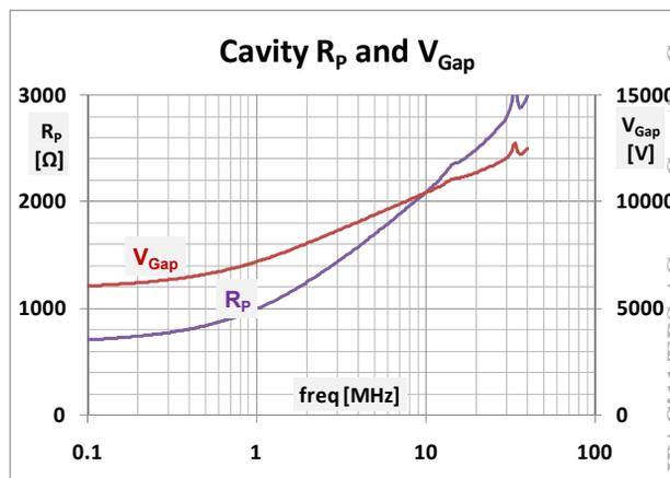
Figure 7: Expected cavity losses and voltage vs. frequency.
