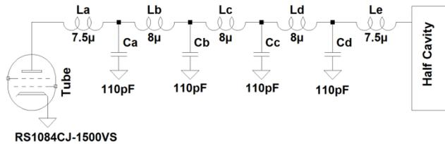
Figure 8: Final stage to cavity compensation network (One of the two push-pull sides).
