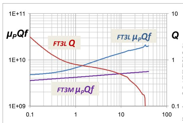
Figure 6: Finemet® FT3L and FT3M measured characteristics.
