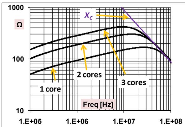
Figure 3: Response of stacked cores.
