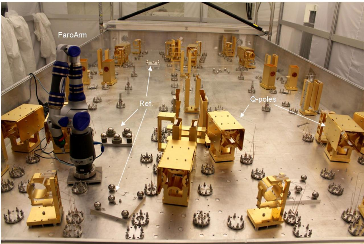
Figure 4: Picture from alignment of the quadrupole doublets showing the portable coordinate machine to the left and some of the reference points used during when the FaroArm was moved from one position to another.
