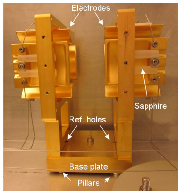
Figure 3: The quadrupole doublet.
