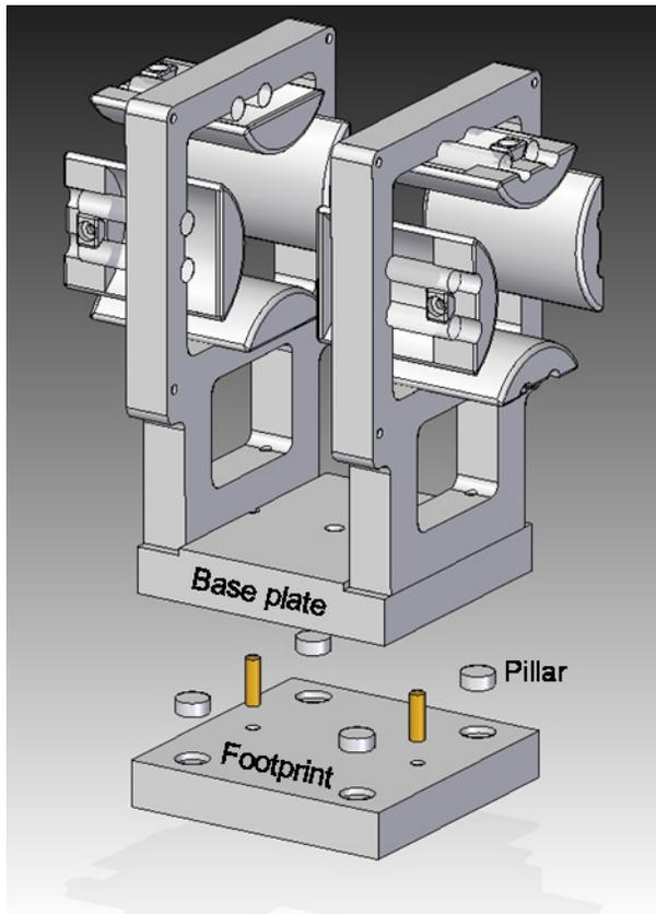
Figure 2: Illustration of the positioning method of the optical elements.
