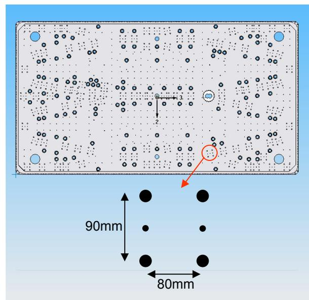
Figure 1: Footprints on the bottom plate.
