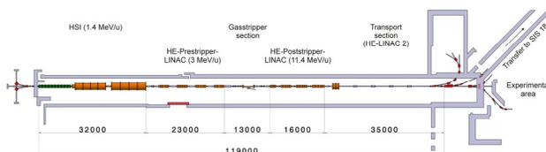
Figure 4: The proposed HE-LINAC (stage 1).
