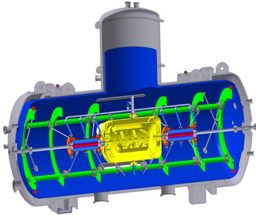
Figure 5: Scheme of the cw-LINAC Demonstrator; the CH-cavity (yellow) is embedded by two sc solenoids (red-orange). A reservoir of liquid helium as well as of liquid nitrogen is reserved (on the top) [5].
