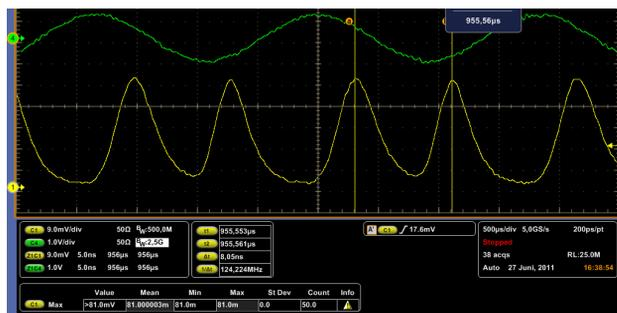
Figure 9: Micropulses of the two beams (yellow). Every second pulse belongs to one channel. The green pickup is the frequency coupled into the resonator.
