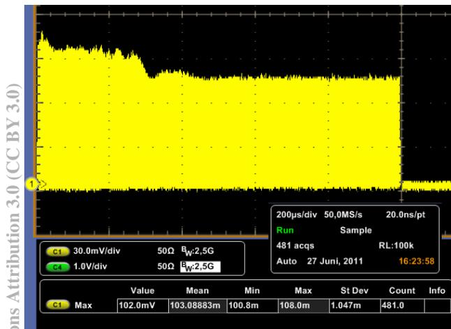
Figure 8: Macropulse of both beams. The pulses are measured behind the new matching section at the crossing point.
