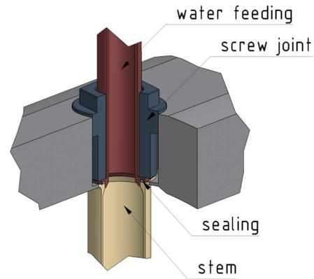
Figure 4: Cross sectional view of detailed stem tank connection
