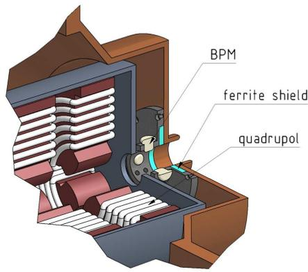
Figure 2: Cross sectional view of a detail of the intertank section with beam position monitors
