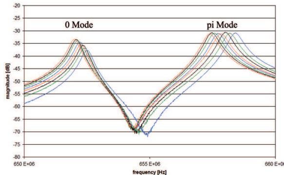
Figure 6: Mode spectrum to show the tuning range of tuner no. 5
