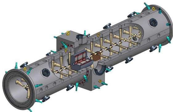
Figure 1: 3D-View of the coupled prototype cavity
