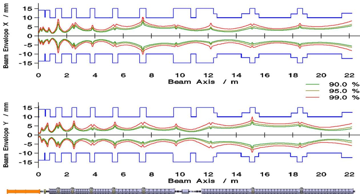
Figure 5: Schematic view of the proton linac with beam envelopes at 80mA, 100% transmission
