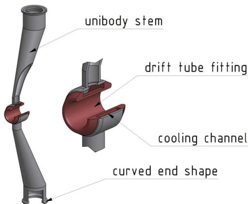
Figure 3: Cross sectional view of an inclined stem with a detail of the drift tube
