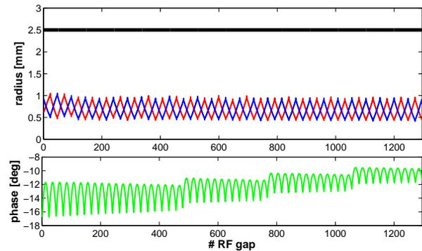
Figure 3: Beam envelope reaching CABOTO acceptance (above) and synchronous phase variation along CABOTO (below). In black, bore hole radius; in red and blue, rms beam size for both transverse planes.
