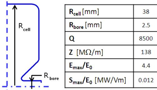
Figure 2: Optimized cell geometry for 150 MeV/u energy particles and corresponding electromagnetic quantities.
