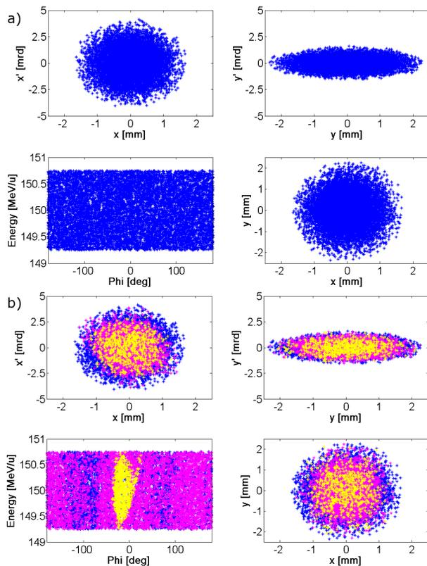
Figure 5: Tracking simulation for CABOTO with a SCENT300-like beam: a) SCENT300-like beam at the entrance of CABOTO; b) In blue, all beam particles; in pink, particles transmitted through the linac; in yellow, those particles transmitted with the appropriate energy.
