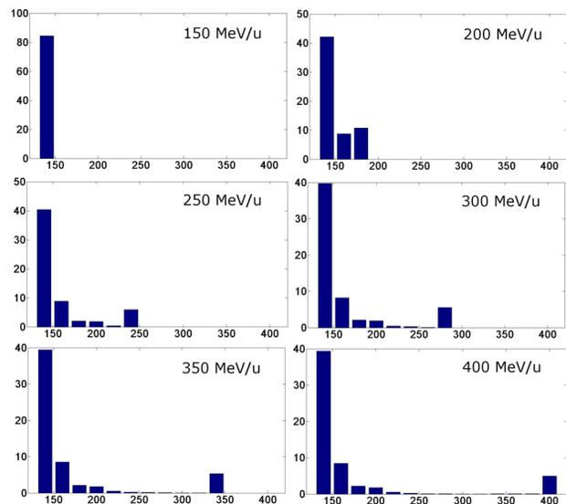
Figure 4: Energy distribution of a beam accelerated by CABOTO to different final energies. The horizontal axes represents the particle energy in MeV/u. The vertical axes is the percentage of particles that have a given energy at the linac exit. A bending magnet and a slit will be used to clean the low energy tail.
