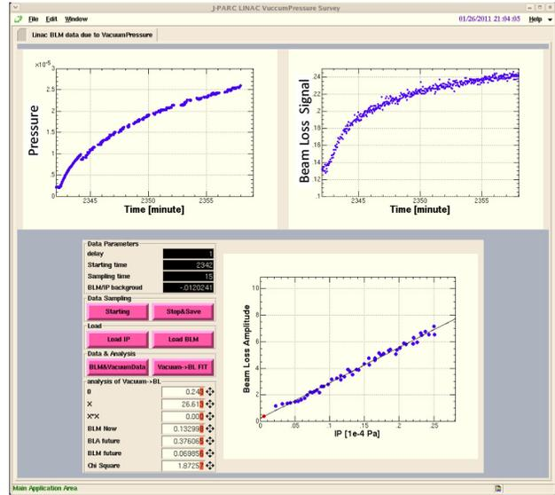
Figure 4: The relation between those two data curves from vacuum meter and BLM.
