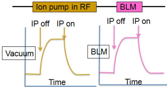
Figure 3: Simply depiction of online experiment study of beam loss due to vacuum pressure control by ion pump.
