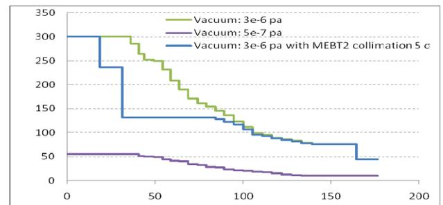
Figure 7: Particle losses in simulations according to different vacuum pressure and case with transverse collimation in MEBT2 section.
