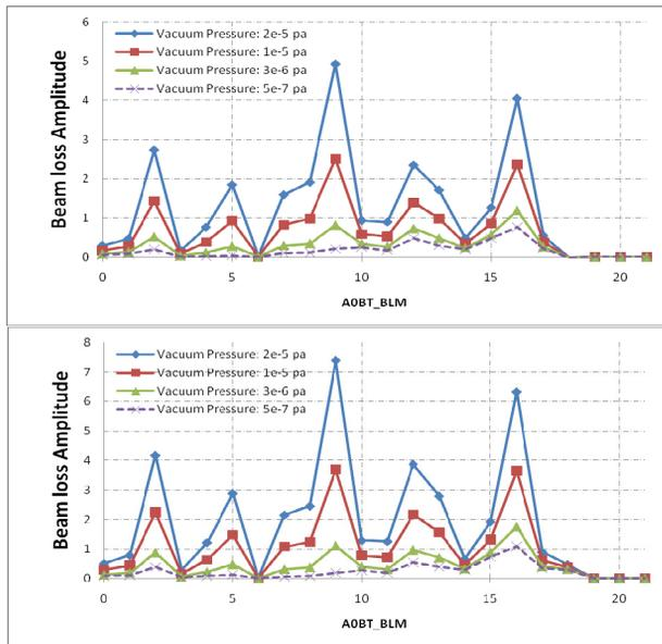
Figure 5: Surmising of beam loss with low vacuum pressure of  $5 \times 10^{-7}$  Pa (Up: 15 mA; Down: 20 mA)
