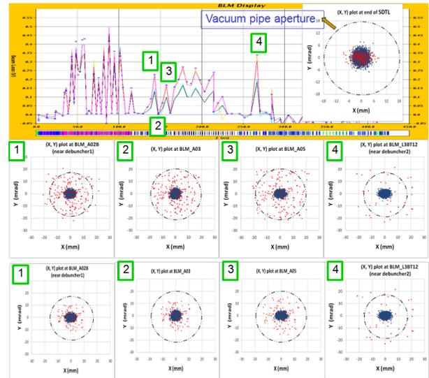
Figure 6: a beam simulation results with residual gas. Beam distributions for 5 place: the end of SDTL, and 4 positions at 4 BLM in future ACS section (blue:  $H^+$  ion; red:  $H^0$ , Up: normal; Down: with MEBT2 collimation)
