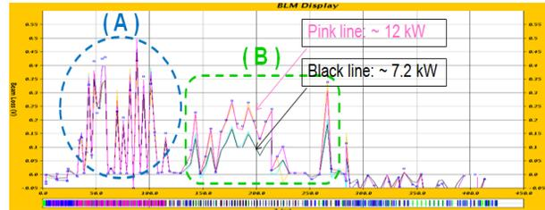
Figure 1: Beam loss of J-PARC linac in normal operation. Beam loss in section A mainly caused by X-ray leaked from DTL and SDTL tanks. Pink: 12 kW beam power from linac & 200 kW from the RCS; Black: 7.2 kW from linac & 120 kW from the RCS.
