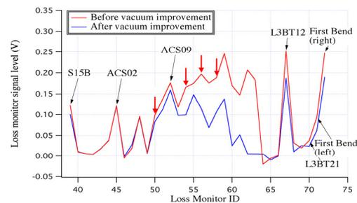
Figure 2: Beam loss profile in the beam transport line after the SDTL exit before and after the vacuum improvement. The red arrows show the locations of NEG pumps in the future ACS section.
