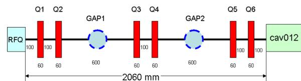
Figure 1: The layout of MEBT for CADS injector-I.
