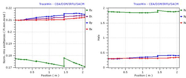
Figure 4: The emittance (left) and halo parameter (right) development in the MEFT line.
