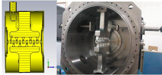
Figure 7: Structure of DTL Tank1.
