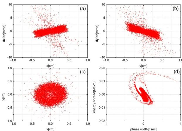
Figure 4: Particle distribution at the exit.
