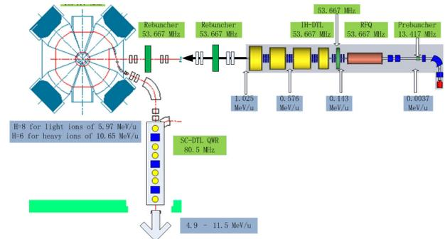
Figure 1: Concept of SSC-LINAC.
