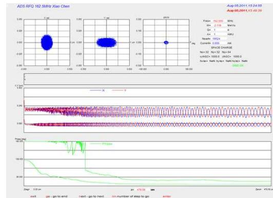
Figure 4: The beam dynamic of RFQ at 10mA beam current.
