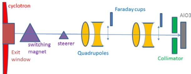
Figure 1: Elements constituting a typical basic beamline. Here an alumina foil (AlO<sub>3</sub>) is located at the end-station.
