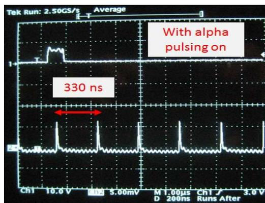
Figure 6: Bunch spacing (330 ns) with the RF deflector.
