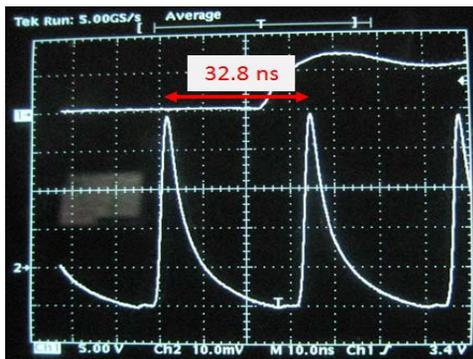
Figure 5: Alpha beam bunch spacing (32.8 ns) without deflectors.
