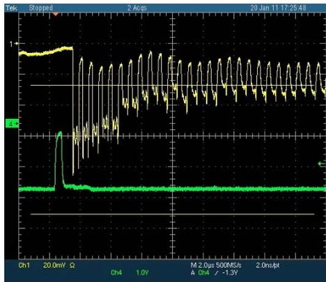
Figure 6: Beam signal of bunch monitor (yellow). Green signal is chopper output signal.
