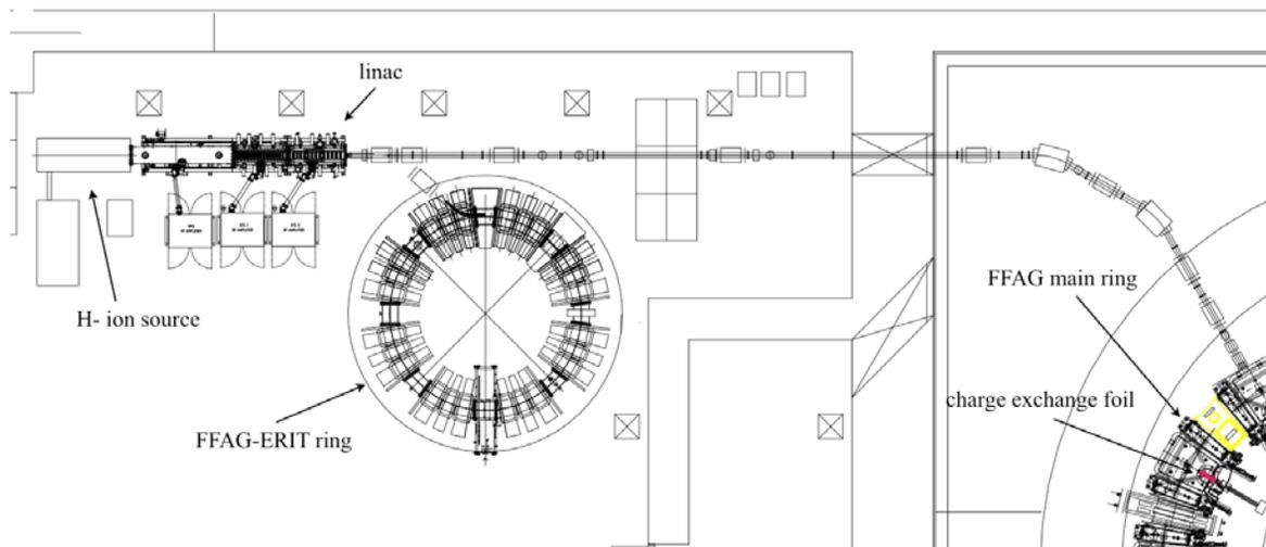
Figure 1: Schematic layout of beam transport line from H<sup>-</sup> linac to FFAG main ring.
