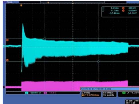
Figure 8: Beam signal of bunch monitor during acceleration (blue). Pink line is signal of output rf voltage.
