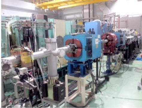
Figure 2: Photograph of beam transport line.
