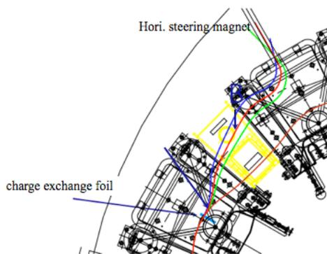
Figure 4: This figure is a H<sup>-</sup> injection orbit within main ring (red line). Brown line is a closed orbit of circulating beam.
