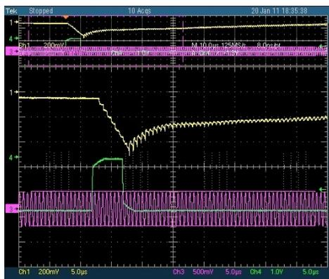
Figure 7: Signal of multi-turn injected beam. Yellow line is circulating beam signal, green line is chopper signal and pink line is signal of output rf voltage.
