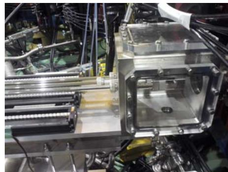
Figure 5: Photograph of installed foil installer machine with mounted carbon stripping foil. The thickness of this foil is  $20 \mu\text{g}\cdot\text{cm}^{-2}$ .
