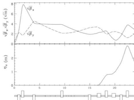
Figure 3: The beam optics of H<sup>-</sup> beam line. (SAD)
