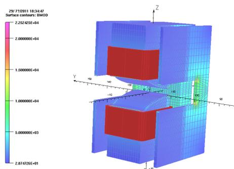
Figure 3: Magnetic field in F magnet (Tosca model).
