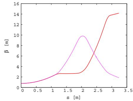
Figure 8: Horizontal (plain red) and vertical (dotted purple) betafuncions in the Straight FFAG line.
