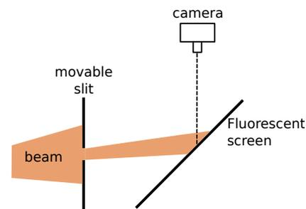
Figure 1: scheme of the emittance measurement system to be installed after the Straight Cell.
