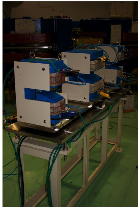
Figure 9: Picture of the straight scaling FFAG magnets prototype.
