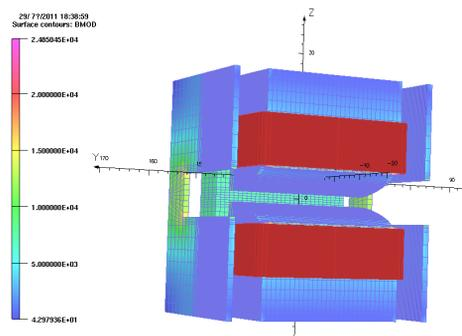
Figure 4: Magnetic field in D magnet (Tosca model).
