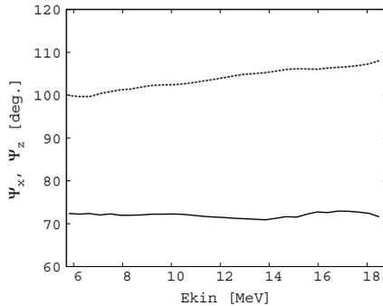
Figure 6: Horizontal (plain) and vertical (dotted) local phase advances versus kinetic energy in the Straight FFAG line.
