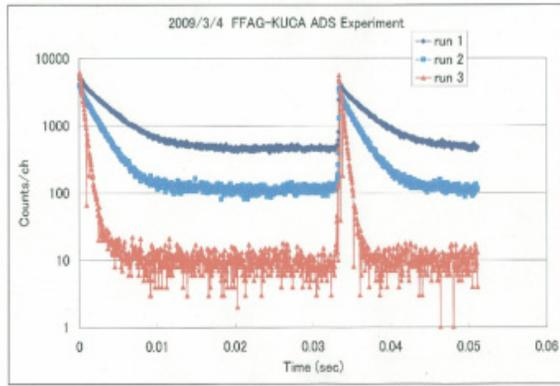
Figure 3: First ADSR experimental result with uranium fuel cores in KUCA.
