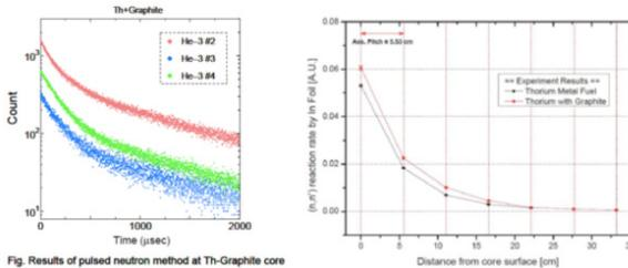
Fig. Results of pulsed neutron method at Th-Graphite core
