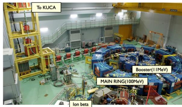
Figure 2: FFAG proton accelerator complex for ADSR study.
