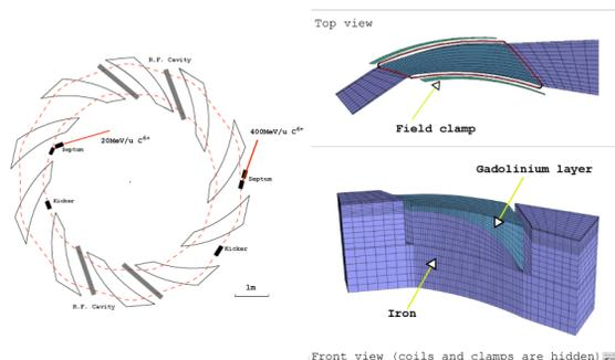
Figure 8: Schematic layout and magnet configuration of superconducting FFAG accelerator for carbon therapy.
