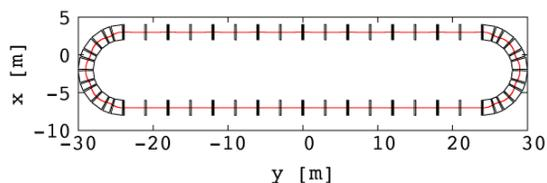
Figure 6: Schematic layout of muon FFAG storage ring with zero-chromatic straight sections.
