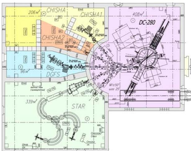
Figure 5: The layout of the DC-280 cyclotron complex.
