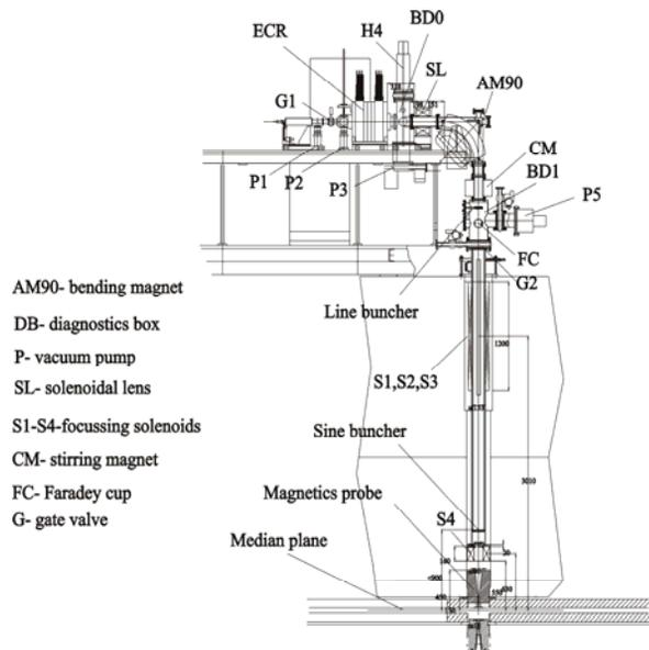
Figure 3: Scheme of the U-400R axial injection system.
