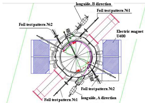
Figure 1: The scheme of beam extraction from U400R.
