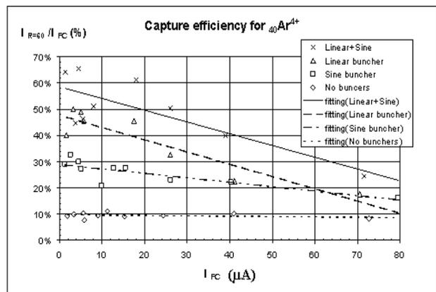
Figure 4: The efficiency of beam capture into acceleration as a function of injecting beam current and bunching effect.
