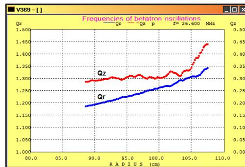
Figure 3: Dependence of betatron tunes on the radius for the optimized sector spiral angle.
