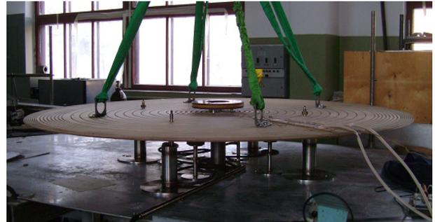
Figure 6: Measurement disk with search coils for the C235-V3 cyclotron.
