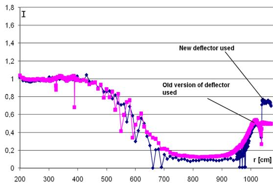
Figure 2: Proton beam extraction in the C235 cyclotron with the old IBA deflector and the new electrostatic deflector.
