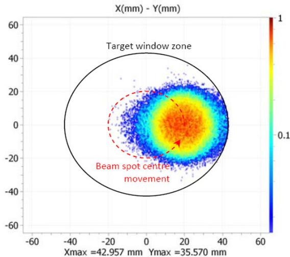
Figure 3: Beam spot movement on target
