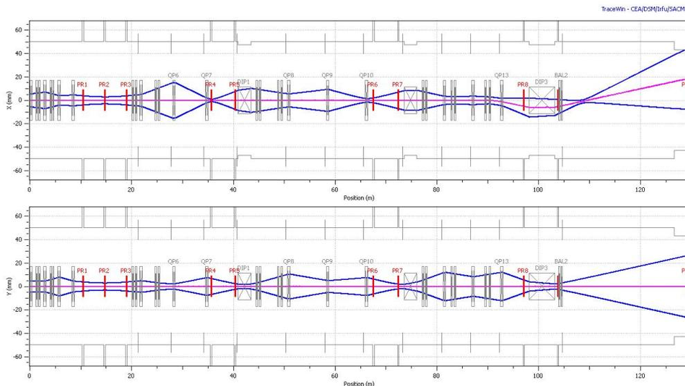
Figure 2: Nominal beam envelopes through the beam line (99%, 3sigma envelopes)
