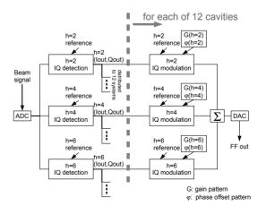
Figure 1: Block diagram of the multi-harmonic feedforward system.
