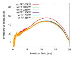
Figure 5: Comparison of  $\phi_s$  without and with feedforward.
