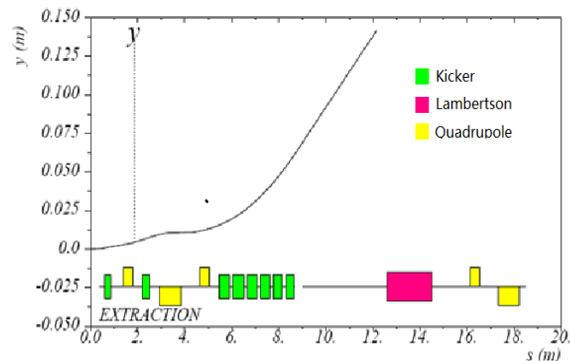
Figure 5: The layout of final extraction scheme.
