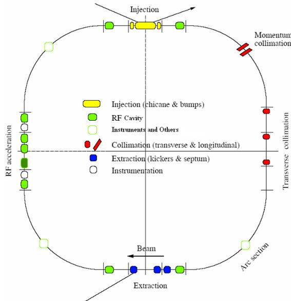
Figure 1: The sketch map of dedicated functions distributed in the different sections of ring.
