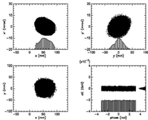
Figure 3: Beam distribution in phase spaces at injection end by an x-y anti-correlated phase space painting.
