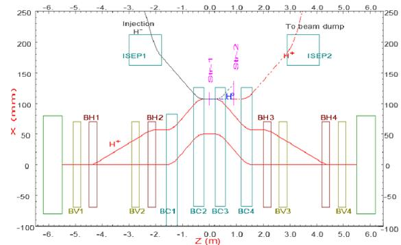
Figure 2: Injection component layout. BC1~BC4: Fixed orbit bump magnets, BH1~BH4: horizontal painting bumpers, BV1~BV4: vertical painting bumpers, ISEP1&2: septum.
