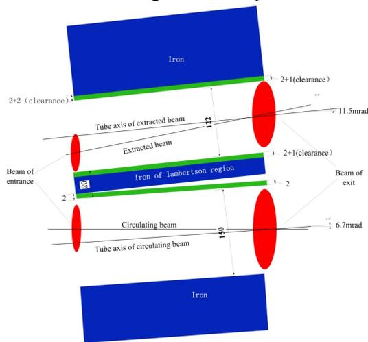
Figure 6: Schematic diagram of the Lambertson septum magnet cross section along the beam.
